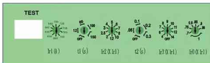
800, I_n=800A Electronic tripping device
